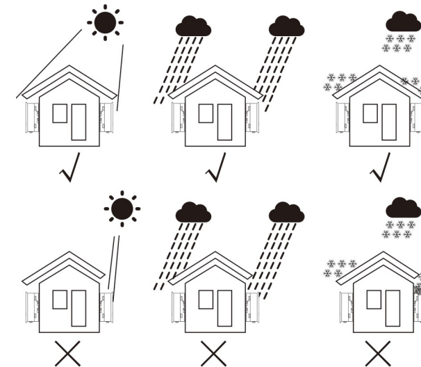
Figure 5.1 Recommended Installation locations
